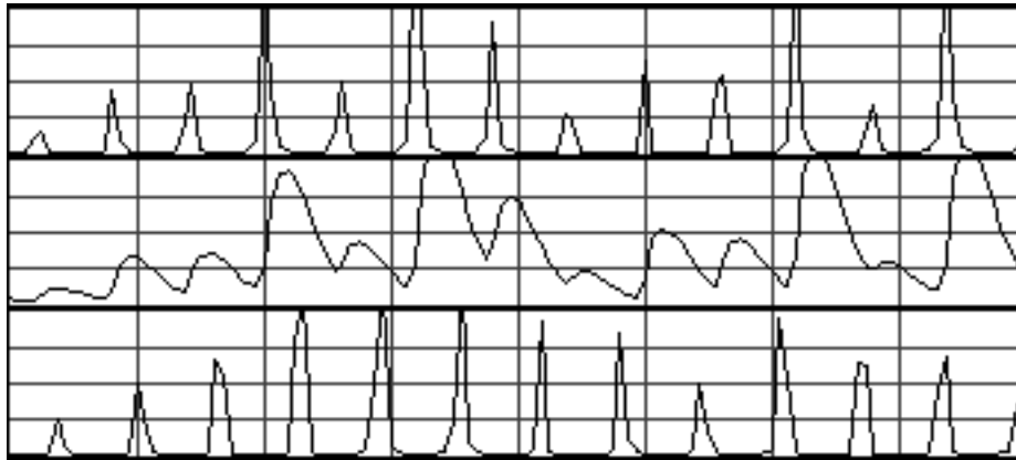
figure 9: top: notched amplitude spectrum of Sound A middle: Sound A's amplitude spectrum smoothed to reduce notches (zeros) bottom: notched spectrum of Sound B
